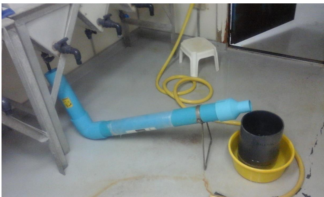
Figure 9. Separation method of Artemia newly hatched nauplii from the cysts using the magnetic separator.
